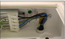
6. Connect the cable to the terminal block.
