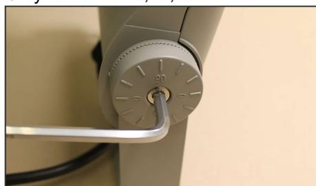
6b. After tilting to the desired position, tighten the screw again.
